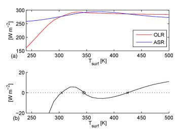
**Figure 8.** (a) OLR, ASR and (b) OLR-ASR for an atmosphere with three thermal equilibria (two stable solutions shown by crosses, one unstable solution shown by the circle). For this example,  $F = 1.025 F_0$  and the  $CO_2$  dry volume mixing ratio was 100 ppm.
