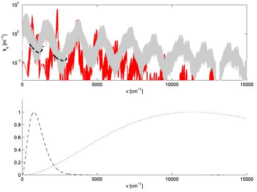
**Figure 4.** (a) High-resolution absorption data for  $CO_2$  (red) and  $H_2O$  (gray) used to create correlated-k coefficients for the radiative transfer calculations. Data shown are for pure gas absorption at 400 K and 0.1 bar. The  $H_2O$  continuum (as defined in Pierrehumbert 2010) is indicated by the dashed black lines. (b) Normalized blackbody emission at T = 400 K and 5800 K (dashed and dotted lines, respectively).
