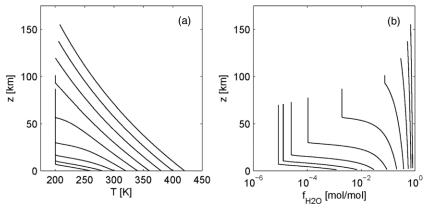
Figure 2. (a) Temperature and (b)  $H_2O$  volume mixing ratio vs. altitude for tests with fixed stratospheric temperature, 1 bar background  $N_2$  and no  $CO_2$ . Profiles finish at a minimum pressure level  $p_{min} = 1$  Pa.
