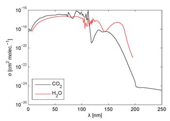
Figure 12. CO<sub>2</sub> and H<sub>2</sub>O absorption cross-sections in the UV used in the model, as a function of wavelength.
