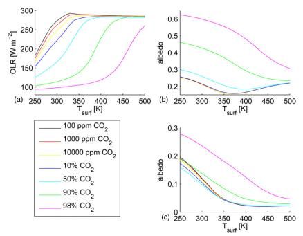
Figure 3. (a) OLR as a function of surface temperature for various  $CO_2$  dry volume mixing ratios, with fixed  $T_{\text{strat}} = 200 \text{ K}$ , 100% relative humidity, and Earth gravity and present-day atmospheric nitrogen inventory. (b) and (c) Corresponding planetary albedo for G- and M-star incident spectra, respectively. (A color version of this figure is available in the online journal.)
