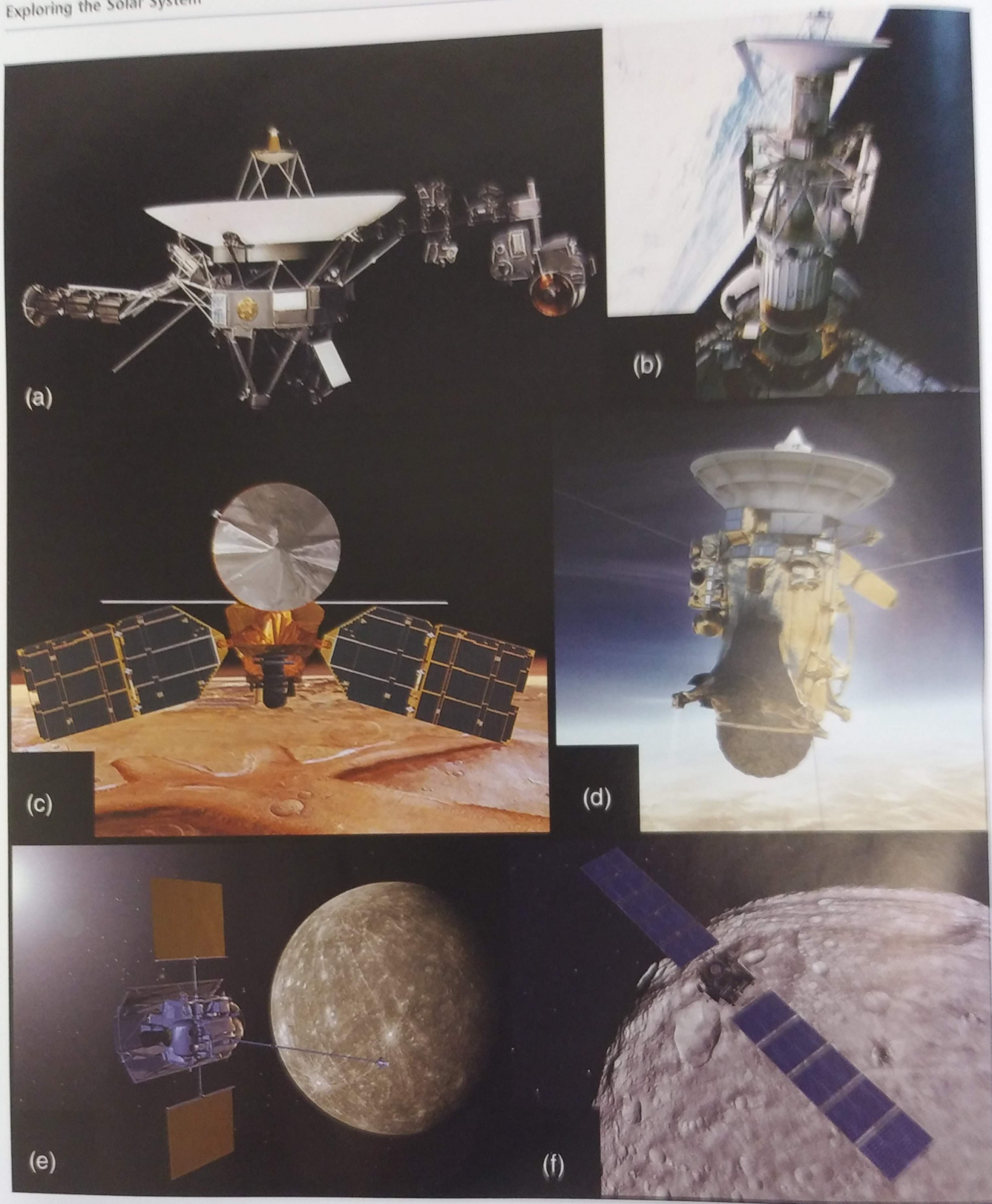
Figure 1.1 A few examples of spacecraft that have flown by or orbited planets and small bodies. (a) Voyagers , which conducted the first exploration of planets of the outer Solar System. (b) Magellan , being launched from the bay of a space shuttle, toward Venus. (c) Mars Reconnaissance Orbiter , mapping the red planet. (d) Cassini , a nuclear-powered probe that explored the Saturn system. (e) MESSENGER , which recently completed its exploration of Mercury. (f) Dawn , with solar panels needed to explore asteroids at great solar distance. NASA images.
