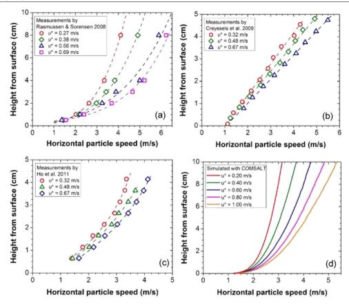
**Figure 14.** Vertical profiles of the horizontal particle speed in steady state saltation from the wind-tunnel measurements of (a) Rasmussen and Sorensen (2008), (b) Creyssels et al (2009) and (c) Ho et al (2011) show that the particle speed converges to a common value near the surface (see also figure 15). This is reproduced by numerical saltation models ((d) and figure 23 in Durán et al 2011a, 2011b). All results are for particle sizes of  $\sim$ 250  $\mu$ m.
