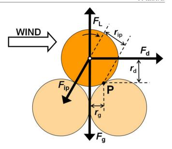
**Figure 4.** Schematic of the forces acting on a stationary sand particle resting on a bed of other particles (after Shao and Lu 2000). Forces are denoted by thick arrows, and their moment arms relative to the pivoting point P are indicated by thin arrows. When the moment of the aerodynamic lift and drag forces exceeds that of the gravitational and interparticle forces, the particle will be entrained into the flow by pivoting around P in the indicated direction.
