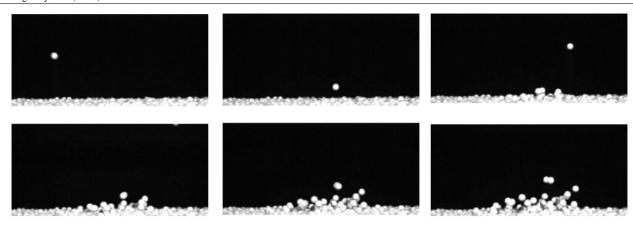
**Figure 8.** High-speed images of the splashing of surface particles by an impacting saltating particle; the time step between two successive images is 4 ms. Reproduced with permission from Beladjine *et al* (2007). Copyright 2007 American Physical Society.
