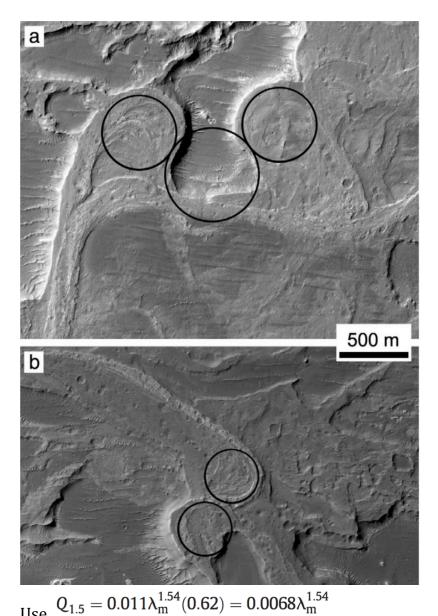
Use  $Q_{1.5} = 0.011 \Lambda_{\rm m}^{-1}(0.62) = 0.0068 \Lambda_{\rm m}^{-1}$ to find bankfull discharge from the two meandering trunk streams shown above. (Remember that wavelength = 2x half-wavelengths). Assume a sediment:water ratio of 1:1000 (by volume) and a lake evaporation rate of 1 m/yr.
