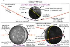
Example geometry of a planetary flyby.
