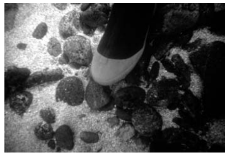
Figure 3.9 Coarse static armor (dark grains) with a partial coverage of finer, mobile sediment (light grains) on the bed of the Trinity River, California, USA. The coarse grains are rendered immobile by the presence of the Lewiston Dam upstream. Image courtesy A. Bartha.
