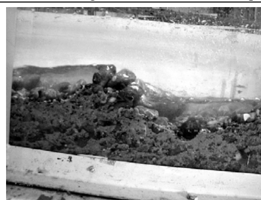
Figure 3.52 Side view of step-pool topography formed in the laboratory. Image courtesy K. Hasegawa.
